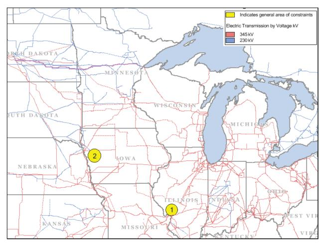
Figure 4.4-1: General location of MTEP12 2017 SUPK baseline generator deliverability constraints
