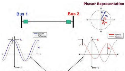
Common Reference Signal at remote locations possible due to GPS synchronization
