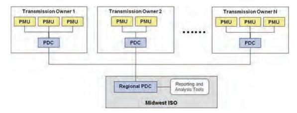
Figure 7.7-2: High-level PMU/PDC framework
