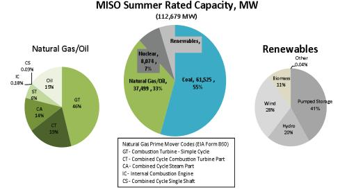
Figure 1.1-4: MISO 2012 Internal Summer Rated Capacity
